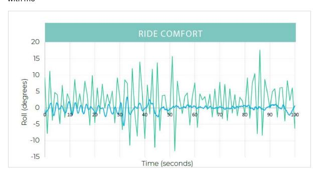
This chart shows the degrees of roll for the Artemis eFoiler®EF12 vessel in blue, and its outboard powered displacement sistership in green. This is measured on the vessels whilst operating at sea via Inertia Measurement Units (IMUs)
